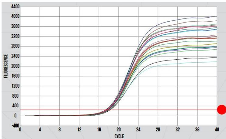
Graph 1: The amplification graph produced by the xpress® from the SYBR-based qPCR detailed.
