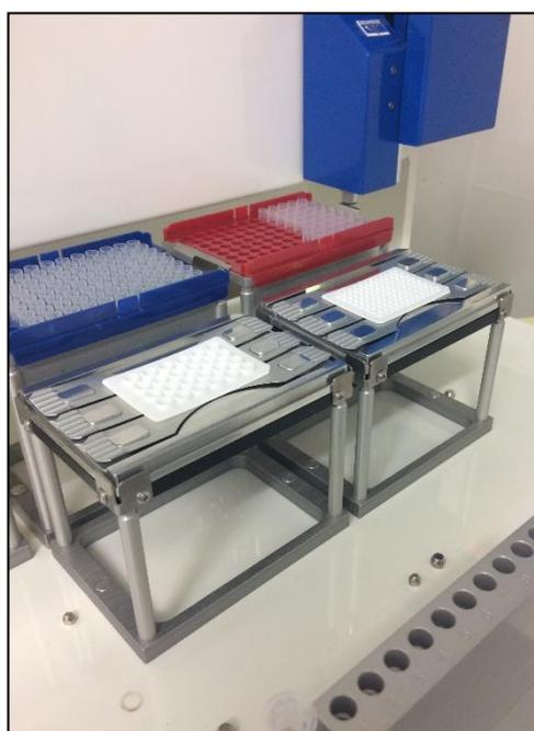
Figure 1: The set up for a 24 well xxplate™ being filled with qPCR reaction mixture by an automated pipetting robot.
