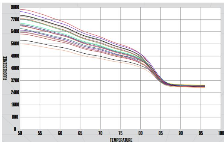
Graph 2: The melt curve produced by the xpress® from the SYBR-based qPCR detailed. The xpress® is also able to plot the temperature against the first derivative of the fluorescence to display the melt peaks.
