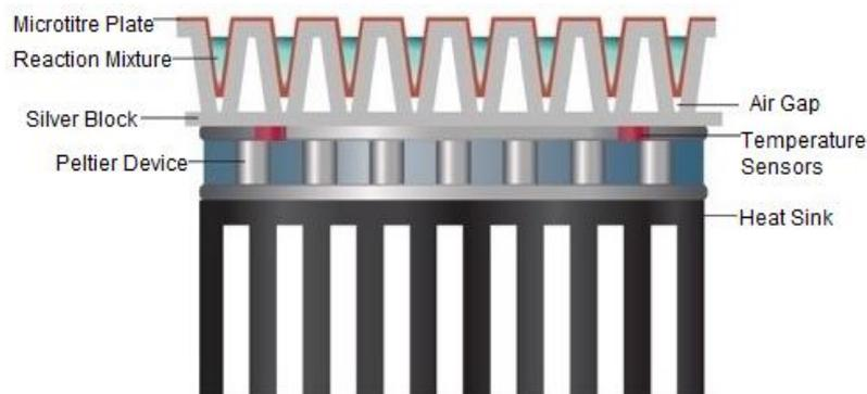
Figure 2. Diagram to show a Peltier device.
