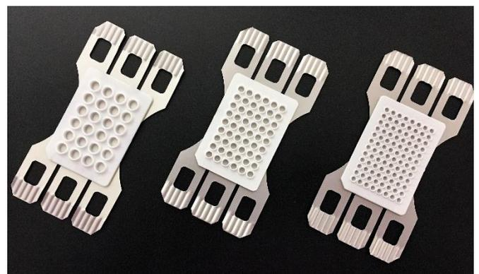
Figure 4. The 3 xplate SBS sizes; 24, 54 and 96 well.
